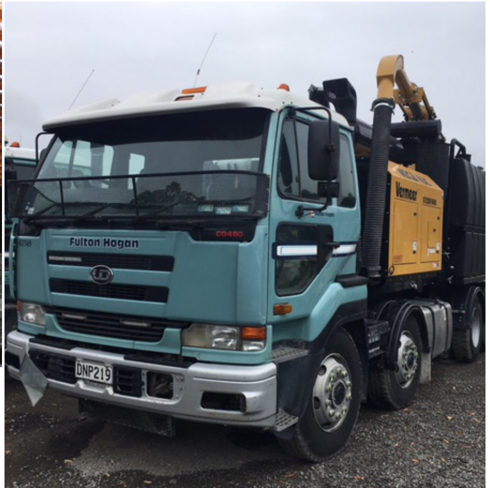
Right: example of a hydrovac.
